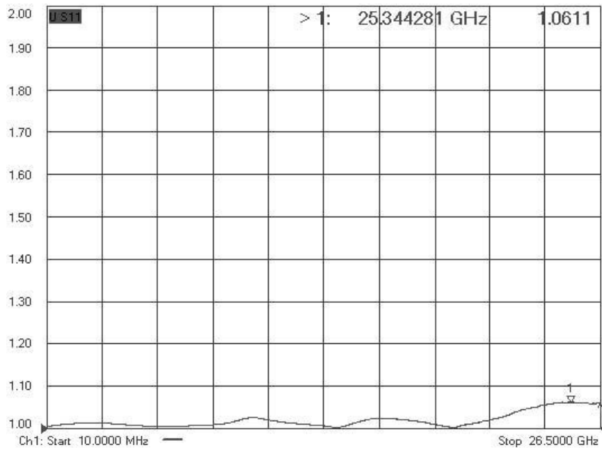
Typical VSWR of 3.5 mm to 3.5 mm adapters, shown from DC – 26.5GHz
