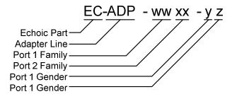
For example, EC-ADP-1818-MF is an Echoic part in the Adapter line where the size of port 1 is 1.85 mm, the size of port 2 is 1.85 mm, the gender of port 1 is male and the gender of port 2 is female.
